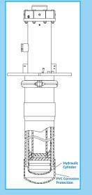
New in-ground hydraulic elevator cylinders are protected from corrosion by encasing the cylinder in PVC.
